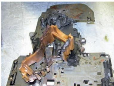
An automatic transmission with heat damage and melted plastic parts.
