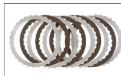
K1 Clutch from DQ250 after 160,000 km
